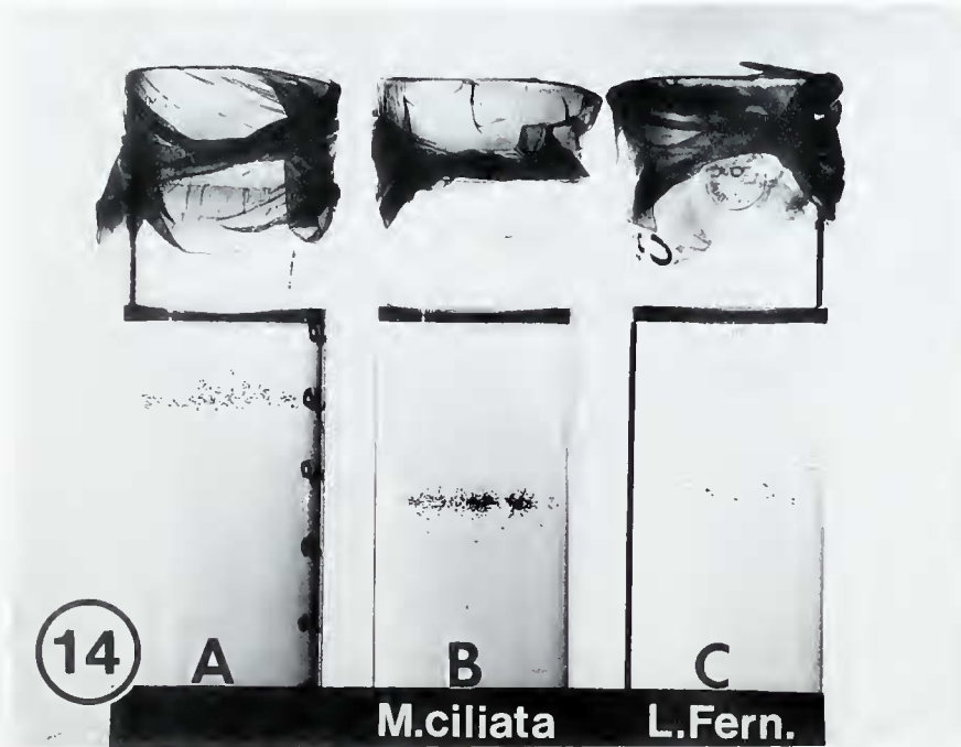
Figure 14. Photograph of eggs of Lepidochitona fernaldi and Mopalia ciliata centrifuged at 400 G's on Percoll gradients in pyrex tubes. A. M. ciliata eggs after 2 min centrifugation. B. M. ciliata eggs after 10 min centrifugation. C. L. fernaldi eggs after 10 min centrifugation.
